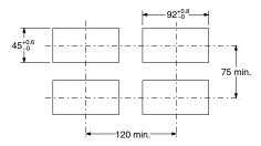
Note: The values above are recommended values. Do not group-mount the meters at intervals less than the recommended ones.
